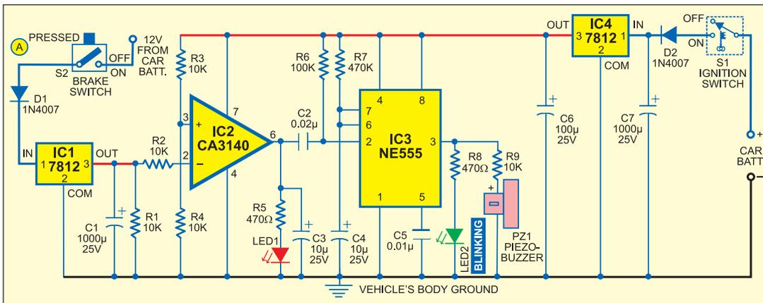
low to switch off the red LED. The low output of IC2 gives a short negative pulse to the monostable through C2 to trigger it. This activates the buzzer and LED2 to indicate that the brake system is working. When there is pressure drop in the brake system due to leakage, LED1
