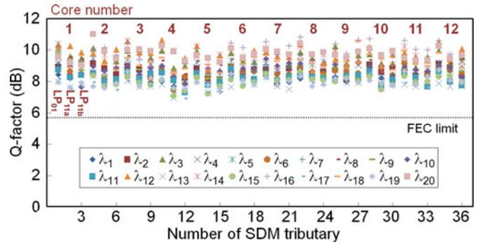
Fig. 9. Measured Q-factor versus the number of SDM tributaries after 40.4 km transmission. The number of SDM tributaries equals  $(n-1) \times M + m$ , where  $n$  is the core number,  $M$  is the total number of modes ( $M = 3$ ), and  $m = 1$  for  $LP_{01}$ ,  $m = 2$  for  $LP_{11a}$ , and  $m = 3$  for  $LP_{11b}$ .
