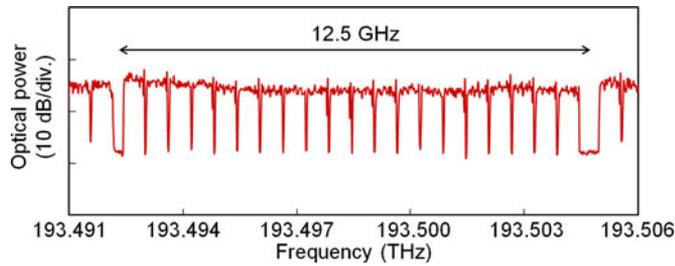
Fig. 8. Signal generated at the Tx, containing 20 independent subcarriers within the 12.5 GHz WDM slot.
