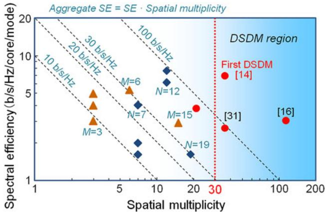
Fig. 2. Spectral efficiency versus spatial multiplicity of SDM-WDM transmission experiments ( $N$ : Number of cores,  $M$ : Number of modes).
