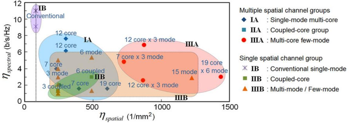
Fig. 4. Spatial and spectral efficiencies of SDM-WDM transmission experiments from various categories of the SDM transmission matrix.
