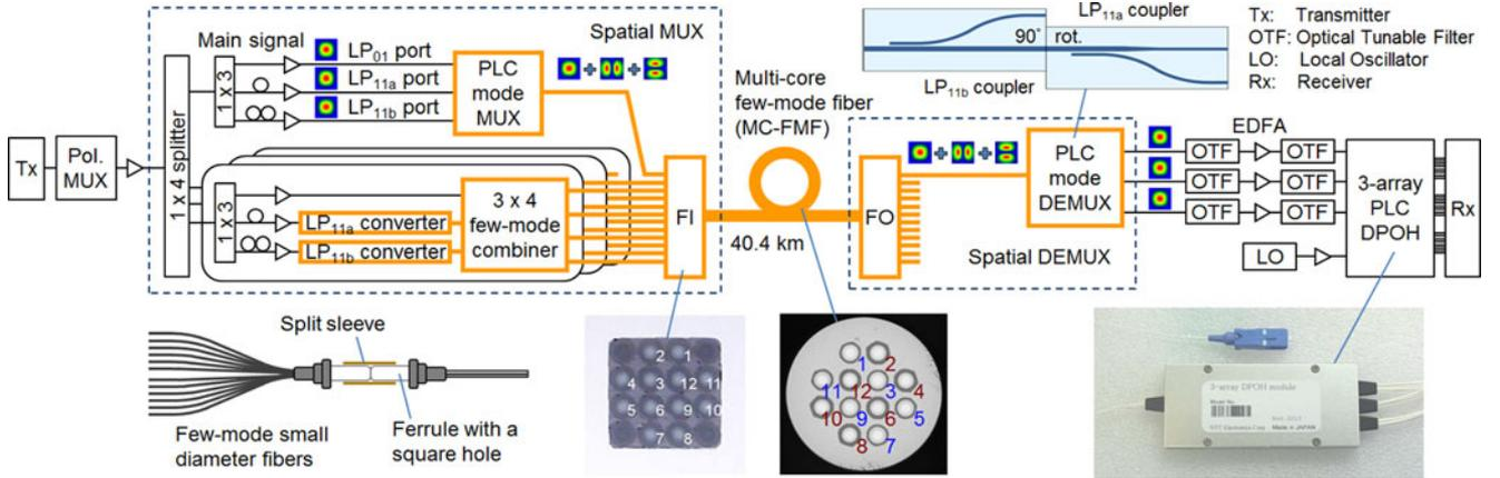
Fig. 7. Experimental setup of the first DSDM transmission experiment.
