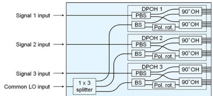
Fig. 6. Schematic diagram of 3-array integrated dual polarization coherent receiver front-end circuit (PBS: polarization beam splitter, BS: beam splitter, OH: optical hybrid, and DPOH: dual polarization optical hybrid).
