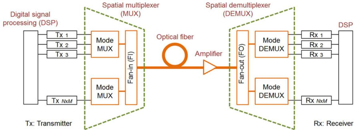
Fig. 5. Example configuration of a DSDM transmission system. The system includes optical fiber, DSP, spatial MUX/DEMUX, integrated devices, and amplifiers for multi-core and/or multi-mode.
