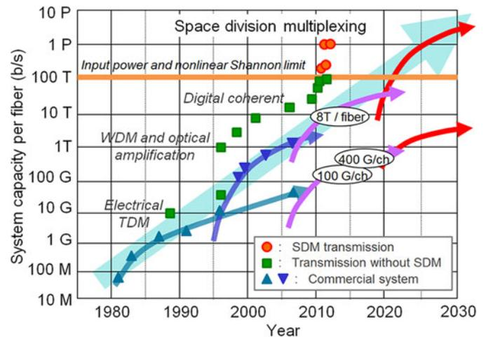
Fig. 1. Transmission capacity per optical fiber in research and commercial systems.
