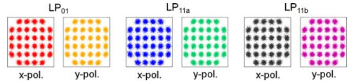
Fig. 10. Measured constellation diagram for core #2, wavelength #10, subcarrier #10 after 40.4 km transmission.
